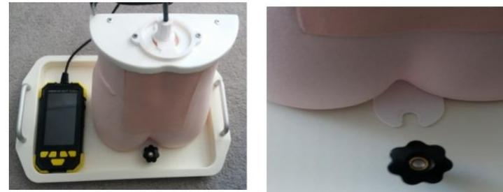
Slide the simulator connector under the rotary knob. Hand tighten the knob to secure the simulator to the tray.
